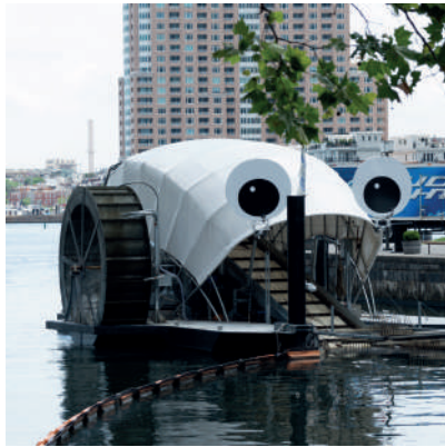
A machine called Mr. Trash Wheel at Baltimore Harbor, USA, uses solar and hydro power to trap trash from the water.
